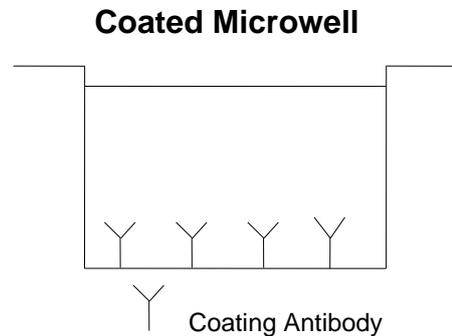
Human VE-cadherin present in the sample or standard binds to antibodies adsorbed to the microwells. A biotin-conjugated anti-human VE-cadherin antibody is added and binds to human VE-cadherin captured by the first antibody.
