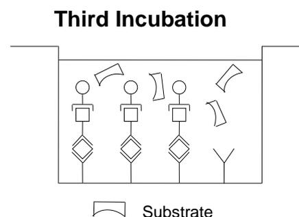
A coloured product is formed in proportion to the amount of human VE-cadherin present in the sample or standard. The reaction is terminated by addition of acid and absorbance is measured at 450 nm. A standard curve is prepared from 7 human VE-cadherin standard dilutions and human VE-cadherin sample concentration determined.
