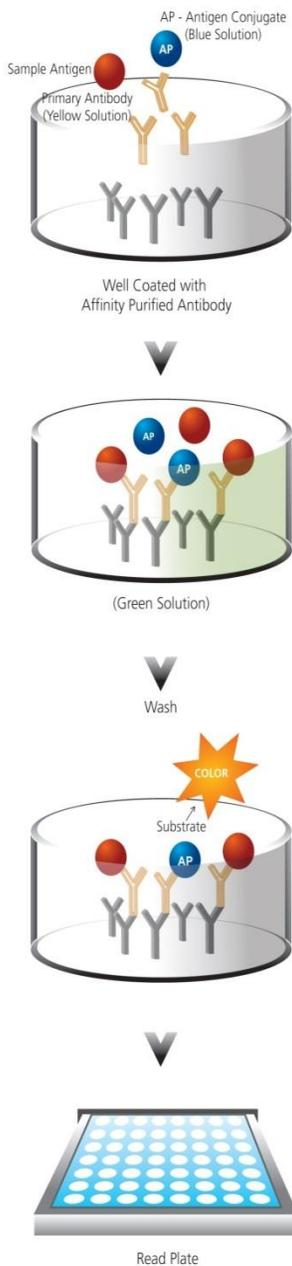
1. Standards and samples are added to wells coated with a GxR IgG antibody. A blue solution of cGMP conjugated to alkaline phosphatase is then added, followed by a yellow solution of rabbit polyclonal antibody to cGMP.
